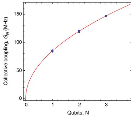
FIG. 5 (color online). Scaling of the collective dipole coupling strength. Measured coupling constants (dots) extracted from Fig. 3 and nine similar data sets and theoretical scaling (line).
