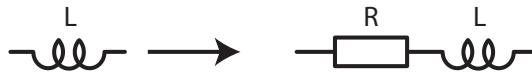
Figure 9: The model for resistive losses in the lumped element transformer consists of this substitution in the original, ideal design.
