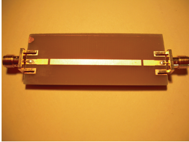
Figure 29: An example of a realized PCB half-wavelength resonator designed for \nu_0=2 GHz. Note the 1mm gap capacitors.
