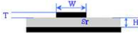
Figure 12: The microstrip transmission line cross section, with center conductor width W , substrate height H , substrate relative dielectric constant \epsilon_r , and center conductor thickness T .
