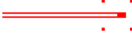
Figure 37: The end of the loaded branch of a CPW impedance transformer. Visible is the 30 \mu\text{m} long end-gap.
