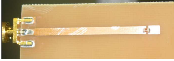
Figure 11: An example of the lumped element transformer on a PC Board. From left to right, note the SMA connector with compensating structure, microstrip line, SMD inductor, and capacitive pad.
