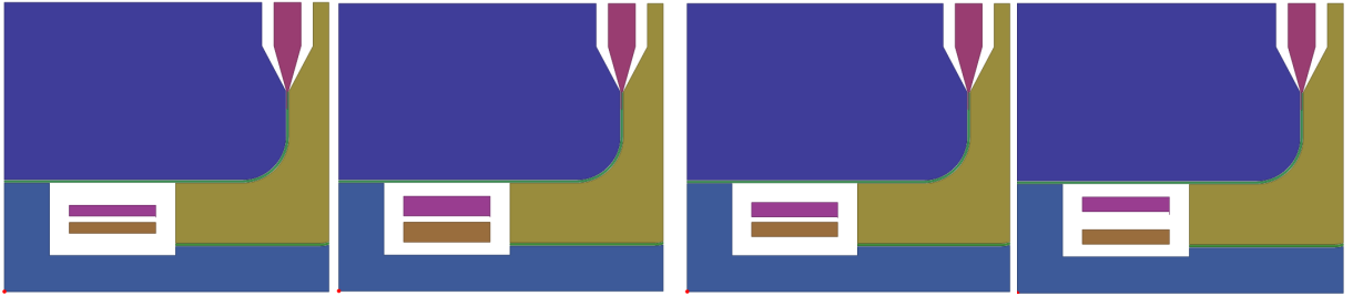
Figure 3: Different geometry parameter settings all with an island length of 480\ \mu\text{m} . From left to right: [width= 60\ \mu\text{m} /separation= 35\ \mu\text{m} ], [width= 110\ \mu\text{m} /separation= 35\ \mu\text{m} ], [width= 80\ \mu\text{m} /separation= 30\ \mu\text{m} ] and [width= 80\ \mu\text{m} /separation= 100\ \mu\text{m} ]
