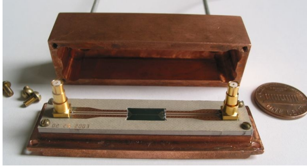
Figure 7: Sample mount made from copper and one cent coin for size scale. Also shown is the chip containing the sample, the PCB and necessary connections.
