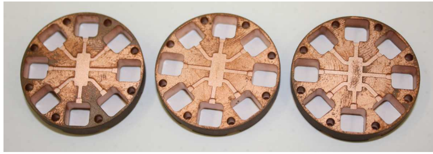
Figure 3.5.: All three covers made from oxygen-free high thermal conductivity 'OFHC' copper, differing only in the height of the cavity above the chip and signal lines. They are from left to right: 0.8mm, 0.5mm and 0.2mm
