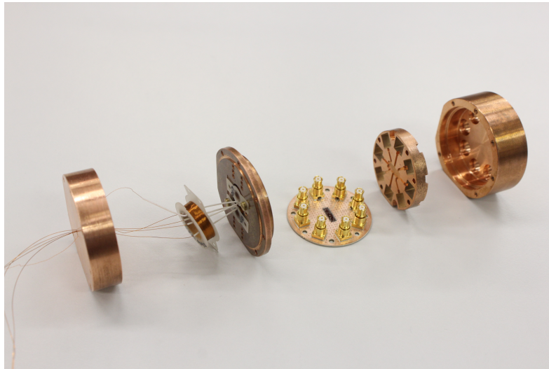
Figure 4.1: Sample holder which is attached to the end of the dipstick. The chip is placed on the copper PCB (third component from the right) and fully enclosed in the copper shielding. This shielding is then fully submerged into liquid helium [20].
