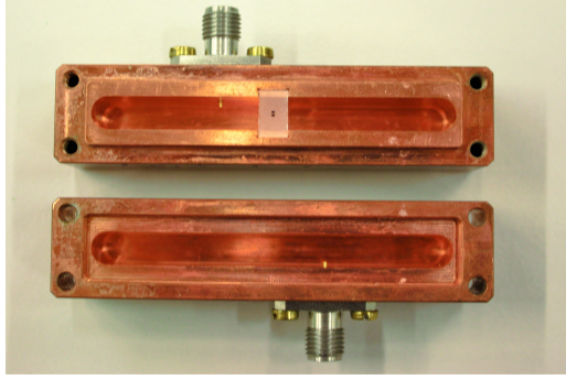
(a) The two parts of the cavity. One can see the mode volume, the sapphire chip where the qubit is attached and the pins of the ports extending into the mode volume.
