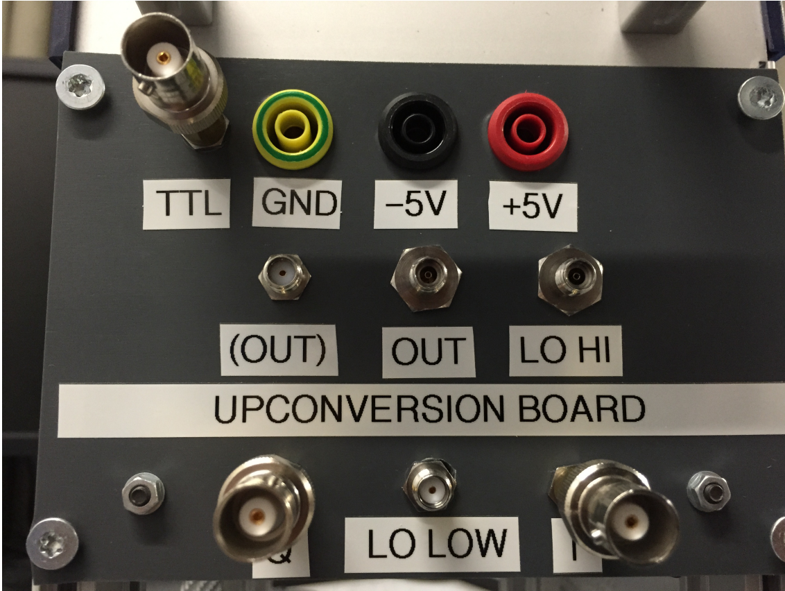
Figure 6: Front panel of the upconversion board. 'LO LOW' and 'LO HI' denote 'LO 1' and 'LO 2' respectively. 'Out' and '(Out)' correspond to 'Out 1' and 'Out 2'. All other labels are identical to Figure 3
