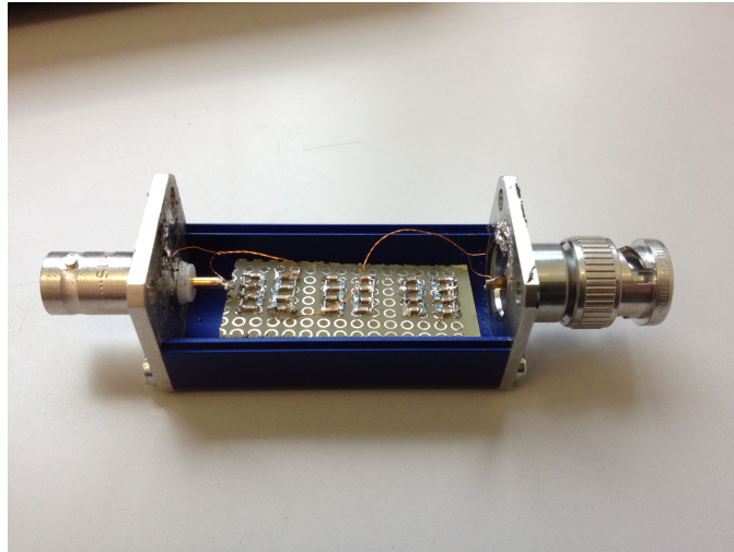
Figure 13: One side of the PCB with the soldered RC-filters, where one filter is connected to BNC.
