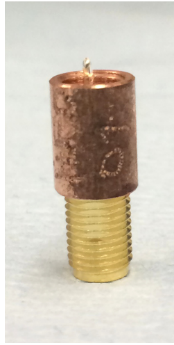
Figure A.3: Center conductor protruding out of LF-TE06 filter body.
