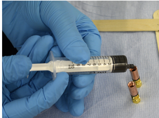
Figure A.6: Image of filters being filled with Eccosorb. Note that filter bodies have just been removed from the hotplate and are still warm.
