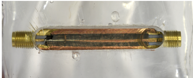
Figure B.4: LF-TE35 01 autopsy image. Cavity almost completely filled with Eccosorb (there is a small void near the left connector) and the center conductors largely remained in the middle of the cavity.
