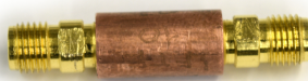
Figure 1: Image of current low-frequency filter (LF-TE10 04). Body length of 15.0 mm, total length of 36 mm.
