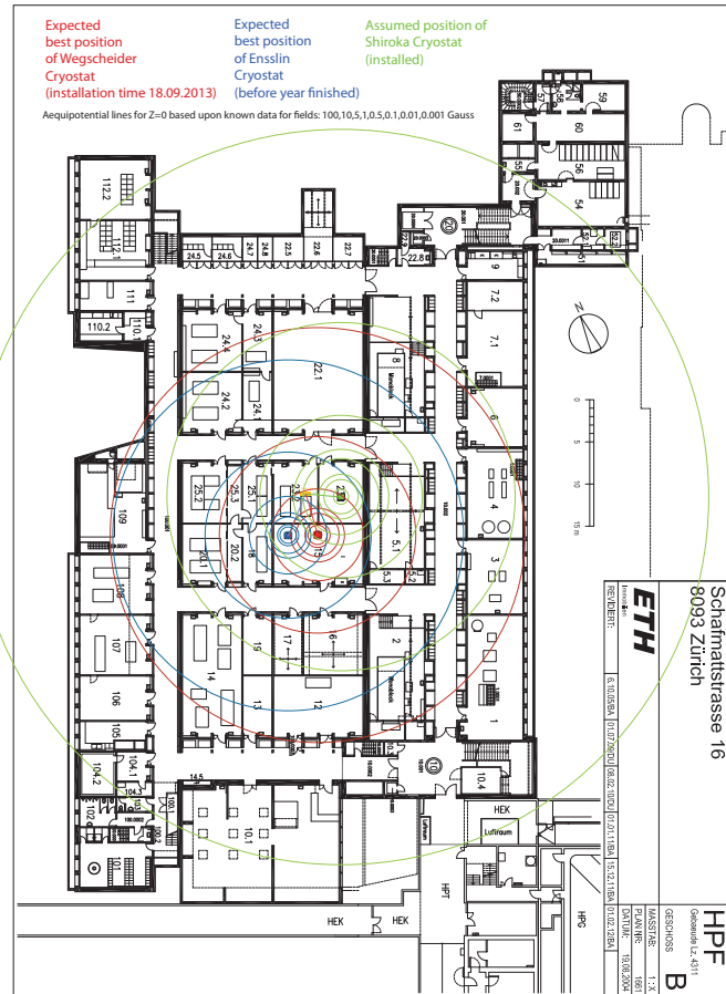
Figure 3: Positions of the magnets of the other groups and estimated field strengths. The position of the experiment is marked with an orange spot.
