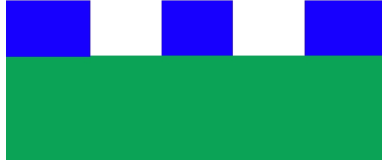
Figure 1: Schematic representation of a coplanar waveguide. The green area represent a dielectric material, the blue area a metal and the white area is air.
