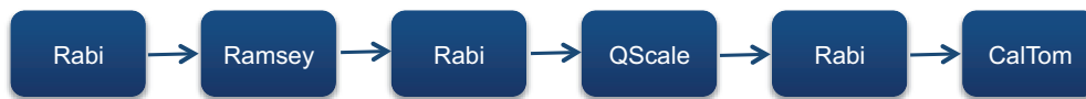
Figure 4.1: Typical sequence of routines for the calibration of the |g\rangle \rightarrow |e\rangle transition.
