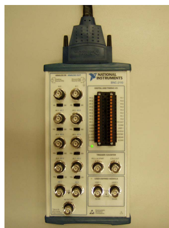
Figure 3.7: Converter card National Instruments BNC-2110, used for applying a bias voltage to the bias box and for reading and digitizing the current and voltage signals from the bias box.
