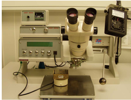
Figure 4.30: Wire bonder West Bond 747677E used for device contacting.
