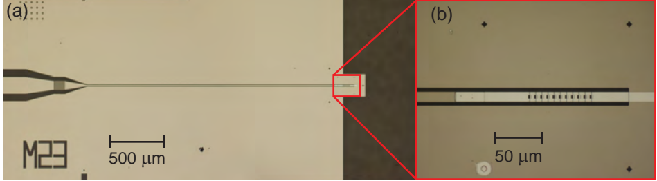
Figure 4.6: (a) Micrograph of one of the used chips with a \lambda/4 -resonator terminated by an array of 11 SQUIDs. (b) Zoom of the SQUID-array.
