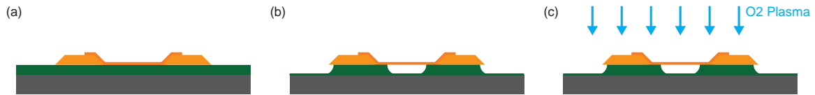
Figure 3.8: Break-junction suspension process: (a) Starting structure. (b) Removal of sacrificial layer, the break-junction acts as an etch mask. (c) Cleaning with O_2 plasma.
