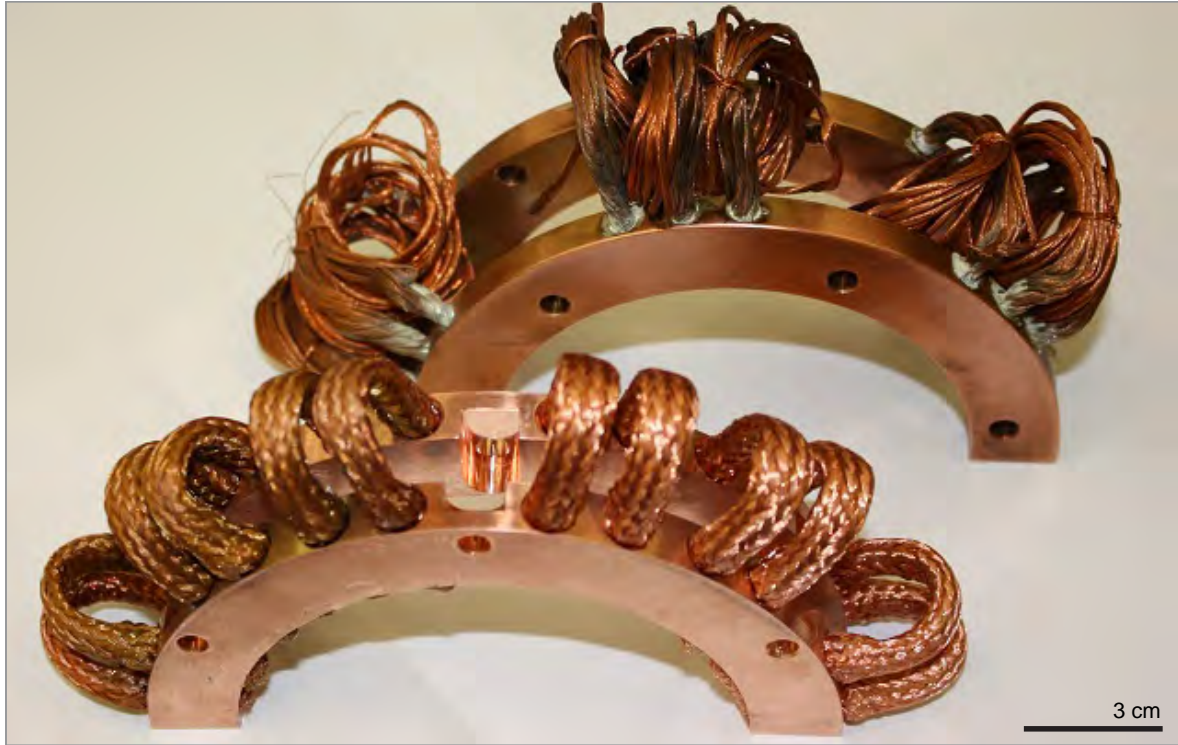
Figure 4.24: Image of the 40 K thermalization half-rings, the initial design is shown in the back, the improved design in front.
