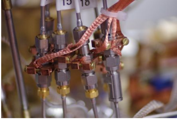
Figure 2.7: To reduce noise, the incoming signal is passed through attenuators which are thermalized to local dilution cryostat temperature using copper connections. This is done at the 4K, 0.1K and base stage.
