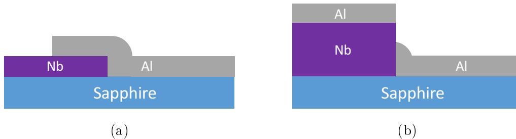
Figure B.3: The schematic for an example of Nb-Al contact. If the thickness of Nb is too large, the connection between evaporated Al parts on Nb will result in discontinuities. (a) The evaporated Al has good step coverage on thinner Nb (b) Bad step coverage for thick Nb film
