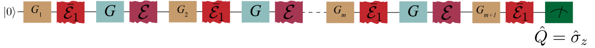
Figure 2.3: One Clifford sequence of length m in the single qubit IRB protocol. This gate sequence is applied to the qubit in the ground state, and the \hat{\sigma}_z operator is measured after the recovery gate, G_{m+1} = (G_m G \dots G G_1)^\dagger . Each Clifford gate G_i in the sequence depicted in light brown is the ideal, unitary implementation of the noisy Clifford gate \tilde{G}_i , that has an associated average error channel \tilde{\mathcal{E}}_1 shown in red. The noisy gate of interest \tilde{G} , whose average error we are interested in finding, is interleaved between every two noisy Clifford gates \tilde{G}_i . \tilde{G} is also decomposed into the perfectly unitary gate of interest G shown in light blue, and its associated error channel \mathcal{E} shown in purple.
