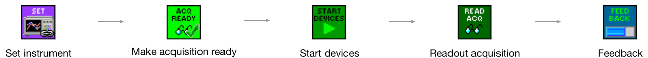
Figure 4.16: A schematic representation of Spot.vi which is the main subroutine of SweepSpot.vi .
