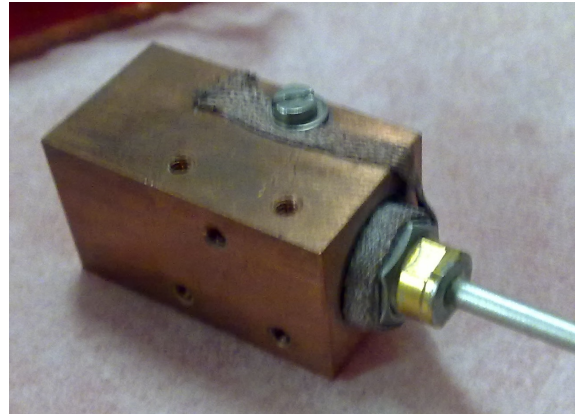
(b) Next the whole construction is pressed into a copper block for thermalization. The end of the copper braid is screwed to the top to prevent the braid from unwrapping itself again.
