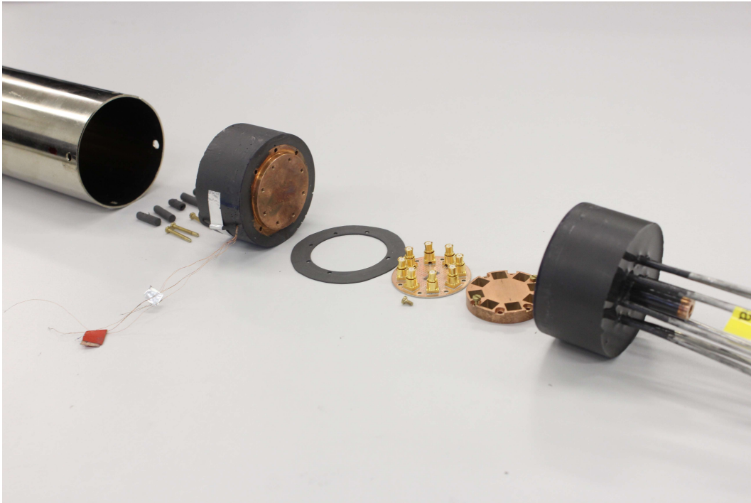
Figure 4.2: A photo of all the assembly components of the Eccosorb box when it is opened, and the magnetic shield into which the box is eventually placed in the DR.
