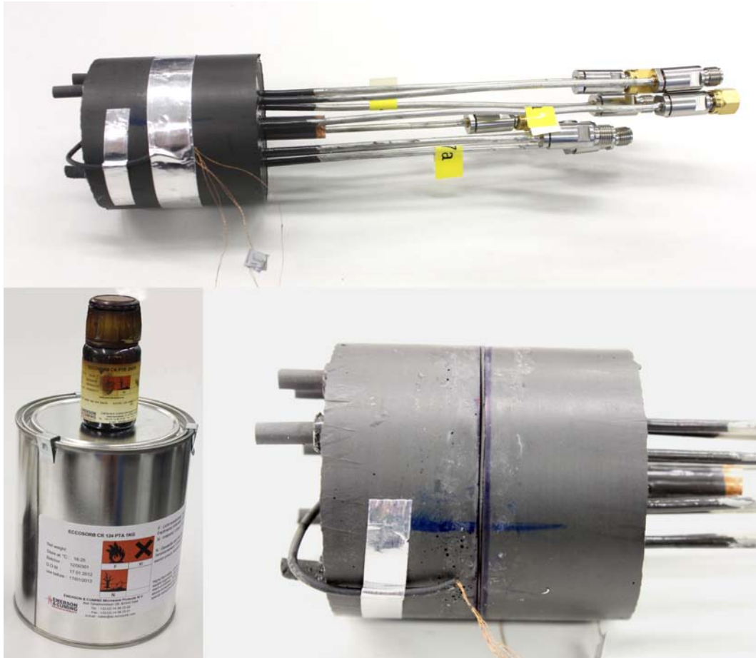
Figure 4.1: (Top) The final Eccosorb box with the 8 microwave cables coming out on top and the three coil wires coming out on the bottom. (Bottom right) A close up view of the two-part box with the o-ring in between. (Bottom left) A photo of the Eccosorb as it is delivered in two parts, the epoxide “resin” in the metal can and the polyamine “hardener” in the small container.
