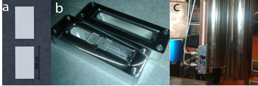
Figure 17: a) A picture of the qubit taken with an optical microscope. The Josephson junction is in the middle of the wire between the two islands. b) Two qubits on separate chips mounted in a 3D cavity. c) A 3D cavity mounted in a dilution refrigerator.
