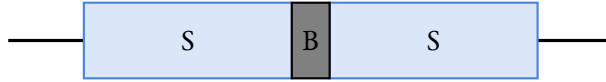
Figure A.3: Basic diagram of a Josephson junction. Two superconducting regions (S) are separated by a thin barrier region (B). For our qubits, these barriers are a thin layer of insulator.
