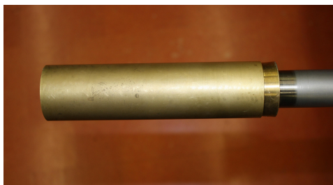
Figure 3.6: The sample holder covered by a metallic cylinder. The cylinder protects the sample from direct contact to the helium and thus allows so to heat the sample to the desired temperature
