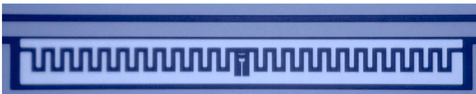
Figure 2.13: Optical microscope picture of a transmon qubit fabricated in the clean room facilities at ETH Zurich.
