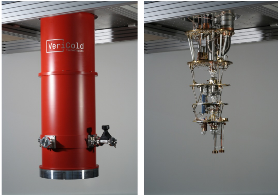
Figure 5.1: The pulsed-tube cooled dilution refrigerator used in the experiments of this thesis: closed state with all thermal and outer vacuum shields (left) and 'undressed' interior (right)
