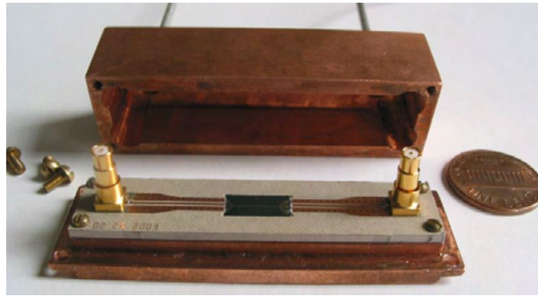
Fig. 3.2: Sample mount made from copper and one cent coin for size scale. Also shown is the chip containing the sample, the PCB and necessary connections.
