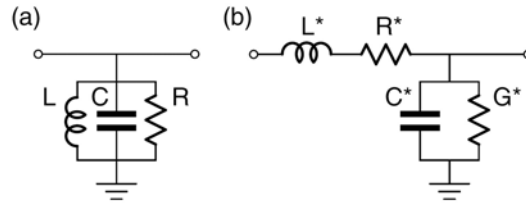
Fig. 2.10: a) Parallel LCR resonator. b) Transmission line model. Figure taken from [68].
