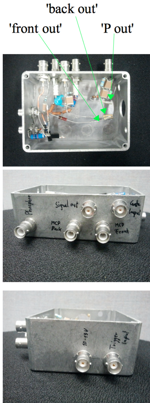
Figure 11: The in- and outputs of the SE on the device. This pictures show the SE without the part Optimization (see Figure 10).
