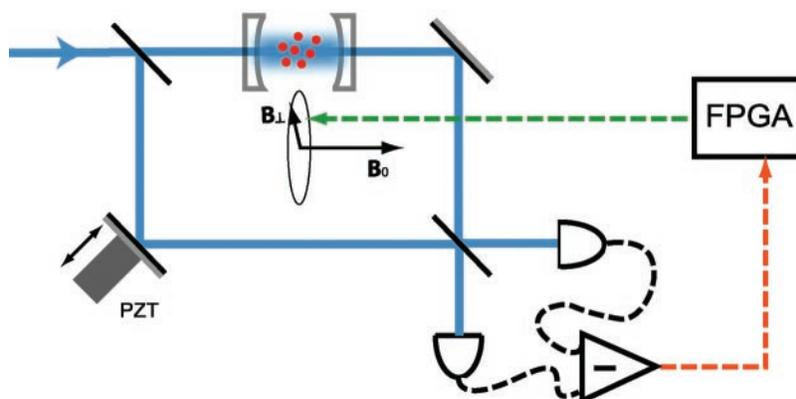
**Fig. 3.** Schematic of an experiment for quantum control of atomic states via strong coupling and real-time feedback, drawn after the scheme proposed in (59). Photocurrent generated by the detection of light transmitted through an optical cavity is processed by a field programmable gate array (FPGA), which sends a real-time feedback signal to influence the quantum state of intracavity atoms via an applied magnetic field  $B$ . PZT, piezoelectric transducer.
