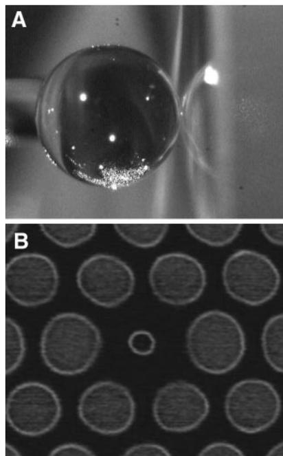
**Fig. 2.** (A) A quartz microsphere dielectric resonator shown next to a glass prism used for coupling via frustrated total internal reflection. (B) Electron micrograph of a photonic bandgap defect cavity formed in an InGaAsP membrane, as described in Painter *et al.* and in Vukovic *et al.*
