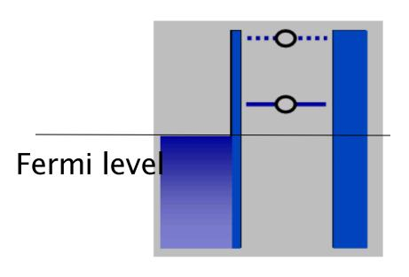
Read-out convert spin to charge then measure charge
