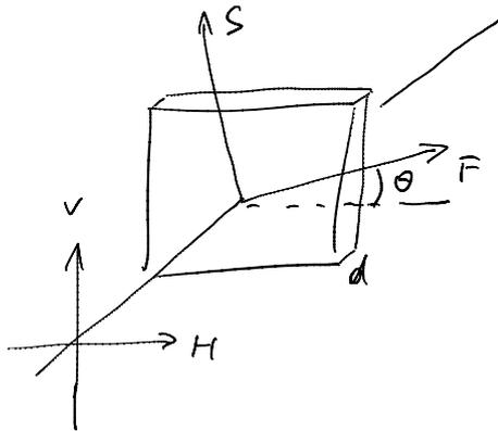
F/S... fast axis (parallel to optical axis)
