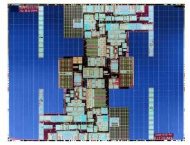
2.000.000.000 transistors smallest feature size 65 nm clock speed ~ 2 GHz power consumption 10 W
