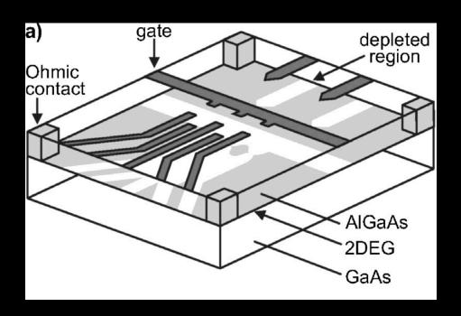
AlGaAs layer doped with Si introduces free electrons which accumulate at the AlGaAs/GaAs interface
