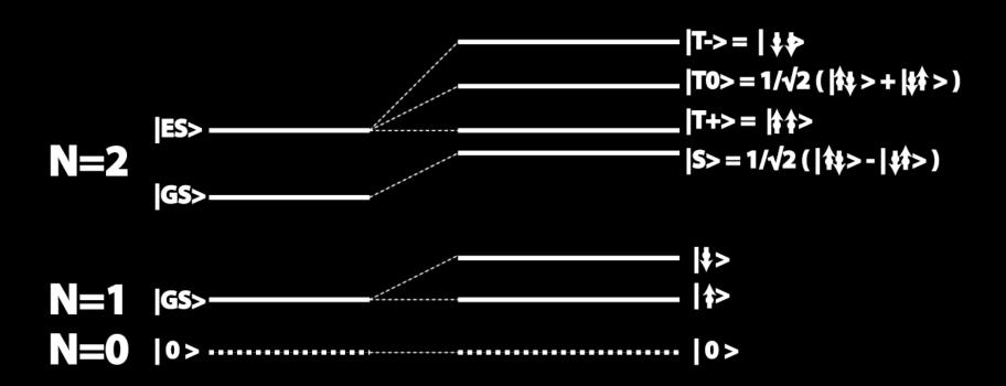
by application of a magnetic field -> Zeeman splitting
