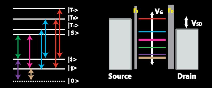
State Preparation: align source potential and transition energy by tuning V<sub>C</sub>
